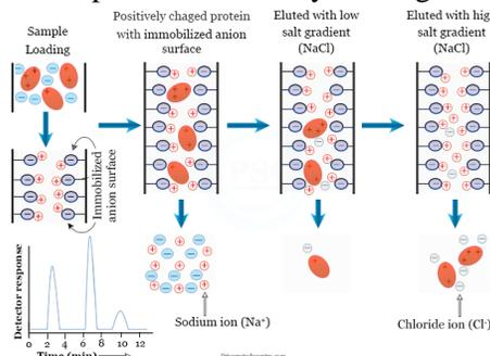
Overall, the working principle of ion exchange chromatography involves the selective binding of analyte molecules to charged groups on the stationary phase, driven by the attraction between opposite charges. This allows for the separation of differently charged or ionizable compounds based on their interactions with the ion exchanger.
