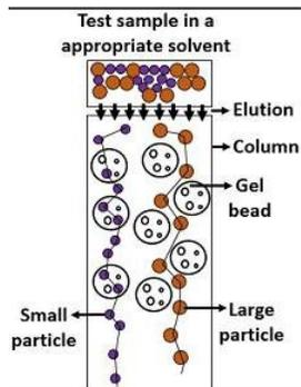
The elution limit is a parameter that affects whether molecules are retained or excluded within the packing material. Those with a larger molecular weight than the elution limit will elute first, while those with a lower molecular weight or size will elute later. In gel filtration chromatography, particles are separated based on their size in this manner.
