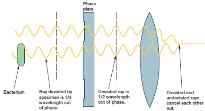
**The Production of Contrast in Phase Microscopy.** The behavior of deviated and undeviated or undiffracted light rays in the dark phase-contrast microscope. Because the light rays tend to cancel each other out, the image of the specimen will be dark against a brighter background.
