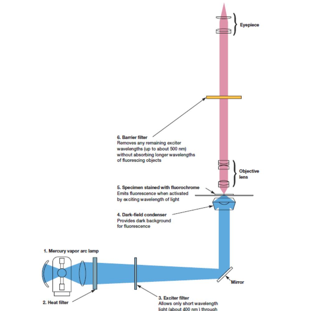
**Fluorescence Microscopy.** The principles of operation of a fluorescence microscope
