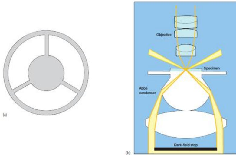
**Dark-Field Microscopy.** The simplest way to convert a microscope to dark-field microscopy is to place (a) a dark-field stop underneath (b) the condenser lens system. The condenser then produces a hollow cone of light so that the only light entering the objective comes from the specimen.
