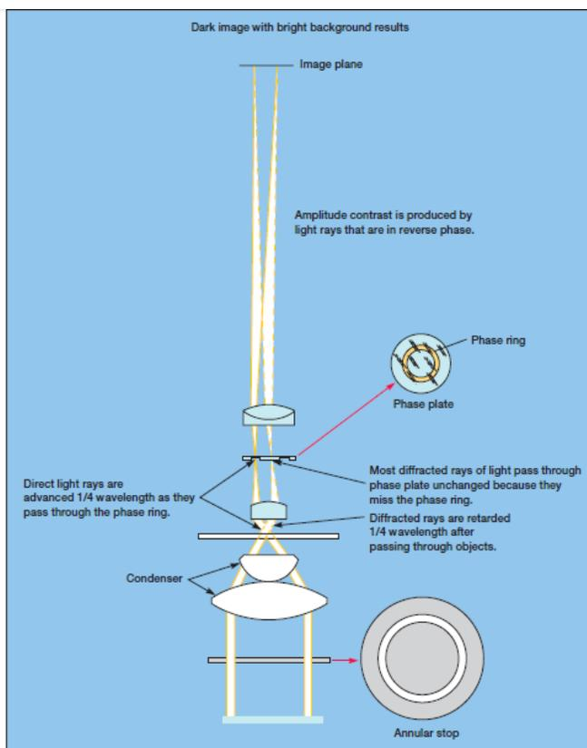
**Phase-Contrast Microscopy.** The optics of a dark-phase-contrast microscope
