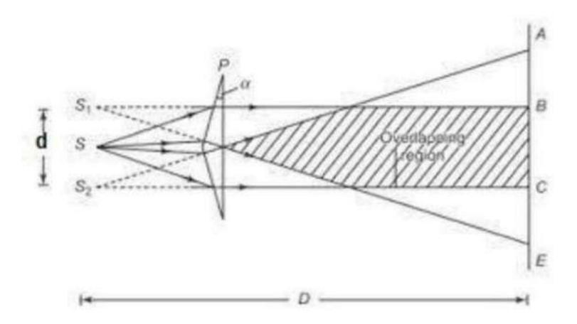
From a Monochromatic source, light through a narrow slit S falls on biprism, which divides it into two components. One of these components is refracted from upper portion of biprism and appears to
