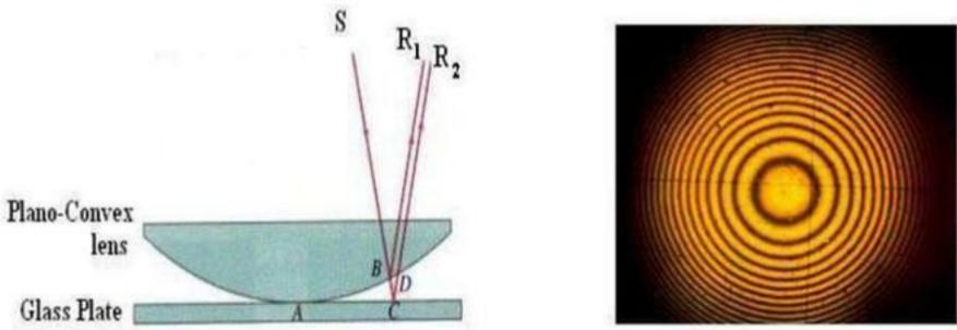
When viewed with monochromatic light, Newton's rings appear as a series of concentric, alternating bright and dark rings, centered at the point of contact between the two surfaces. (fig.)
