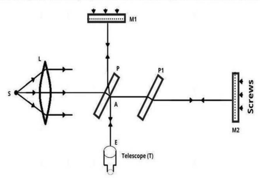
The reflected beam travels towards the movable plane mirror  $M_1$  and falls normally on it and hence it is reflected back to P and gets transmitted towards the telescope T. The transmitted beam moves towards the mirror  $M_2$  and falls on it normally, after passing through a compensatory plate  $P_1$ . It is then reflected back by the mirror  $M_2$  and **retraces** its path. At A on the plate P, it is reflected and enters the telescope T.
